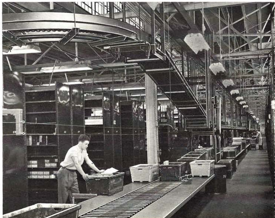
RIGHT: Part of Logan system in wholesale drug warehouse. Live Roller takes tote boxes of filled orders to checkers. Overhead Belt and Roller Conveyor line handles mail and express shipments to an adjacent building.
