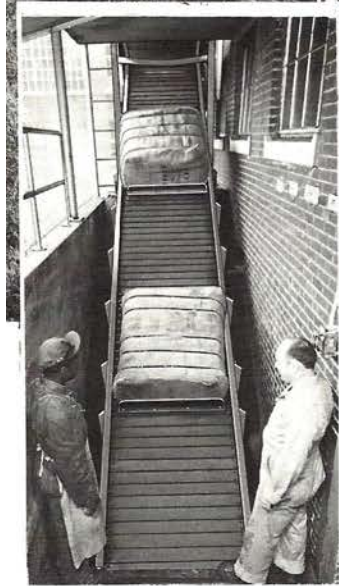
ABOVE: Logan Slat Conveyor handling bales of cloth from basement and first floor storage to finishing department on second floor. View at left shows basement feed end. Platform above serves first floor via hinged slide at entrance to housing. A roller conveyor curve facilitates discharge into building at second floor.
