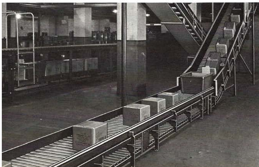
ABOVE: Slat Conveyor used for taking stock from warehouse to shipping room. Handles cases and cartons of all sizes which are loaded directly onto conveyor at any point along the line. The conveyor is installed flush with floor and can be walked on or trucked over, while in motion, without interruption to traffic.
