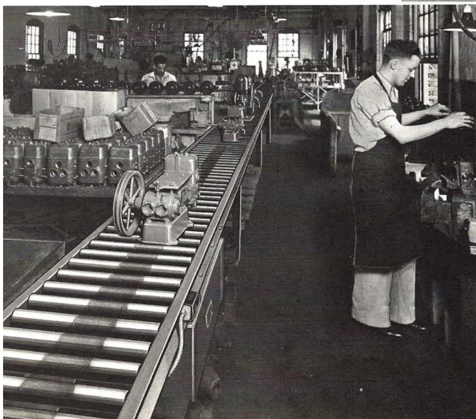
LEFT: This Live Roller Conveyor handles partially assembled gasoline pumps from assembler's benches through testing stations and thence to painting. Units travel at a constant speed and at convenient working height. They can also be stopped on conveyor without excessive wear and tear on the belt.
