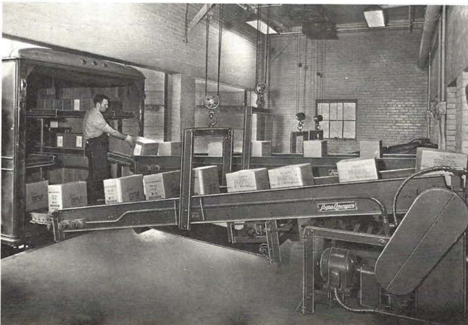
ABOVE: Declining Belt Conveyors with roller cleanouts at discharge for delivery to Roller Conveyor. These Belts and the similar units shown in rear handle cartons of candy to truck loading dock.
