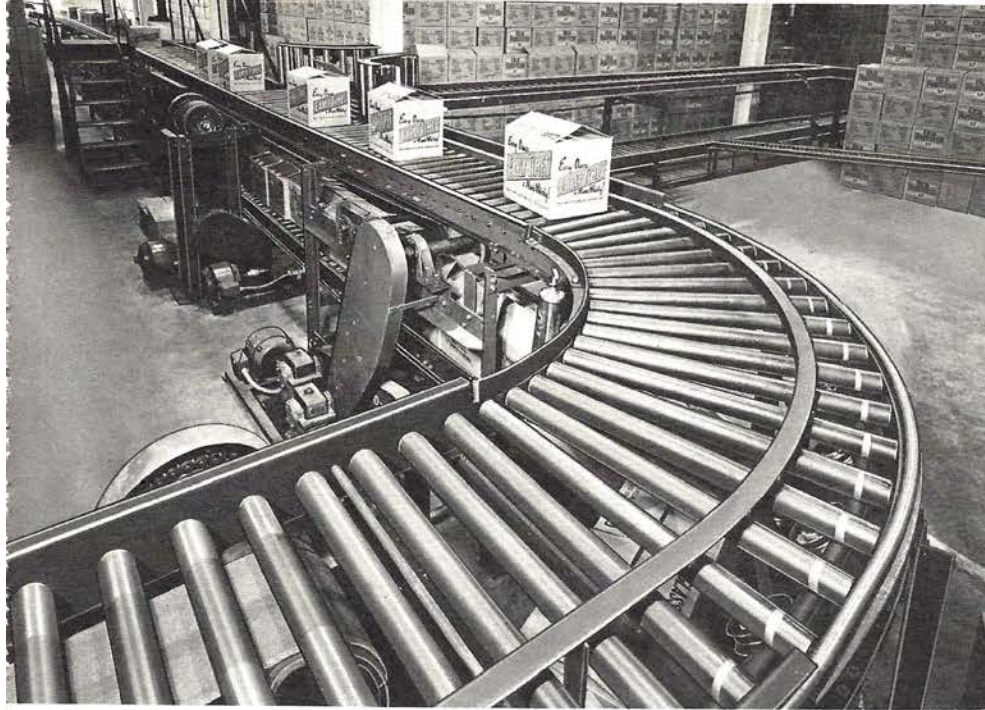
RIGHT: A Live Roller Curve is part of this system which handles metal pails through manufacturing operations. Curve connects two straight Live Roller Conveyors which have belts set to one side for protection from paint on pails. Mule Drives are used to power connecting rolls at both ends of curve. Rolls in curve have flanges which serve as guard rails and as a protection for belt.
