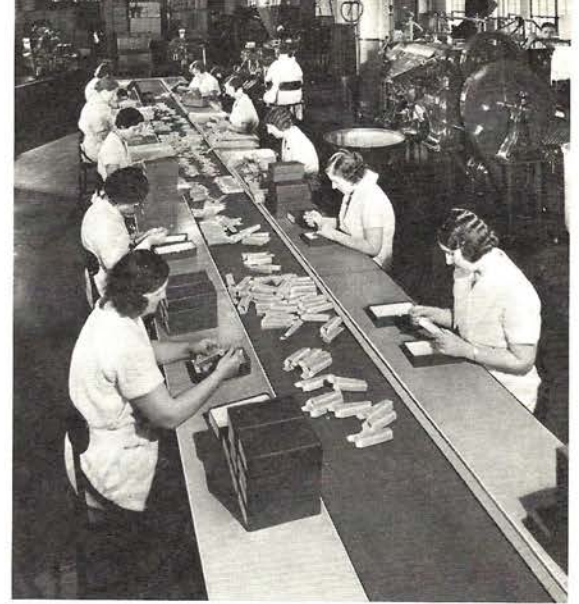
ABOVE: Conveyor Packing Table with slow moving Belt in center and work boards along both sides. This unit speeds packaging of drug products with minimum effort.
