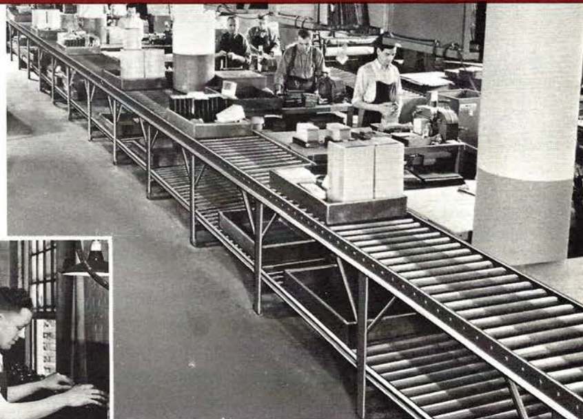
RIGHT: Two-Way Double Deck Live Roller Conveyor in shipping department of a spraying equipment manufacturer. Orders in tote pans are brought in on top deck and pushed out on Roller Conveyor spur lines for packing. Lower deck driven by return run of belt takes the empty tote pans back to stock room.
