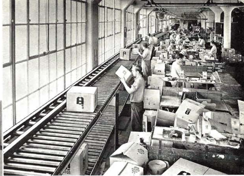
ABOVE: A Double Deck Live Roller Conveyor serving packing department for a manufacturer of perfumes and toilet articles. Both decks operate in same direction. This is accomplished by placing upper run of belt in contact with top surface of rolls and return run with underside of lower deck. The belt is placed along the side adjacent to windows.
