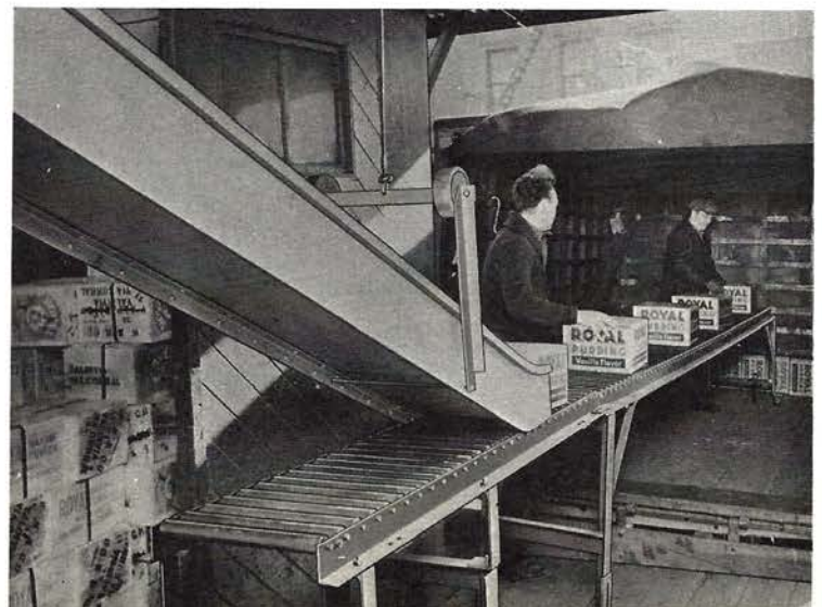
BELOW: Loading trucks for a manufacturer of baking powder and gelatin desserts. Slide is hinged and counterweighted to permit raising when not in use. The Roller Conveyor is mounted on casters and backed into building by degrees as truck is loaded.
