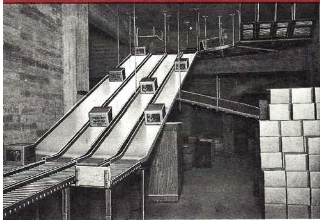
ABOVE: Two groups of straight Steel Slides handling cartons of coffee, syrup, and pancake flour. The cartons pass thru second floor, around Roller Conveyor curves, and down to first floor shipping department. The pitch or slope of Steel Slides can be varied to suit the material handled.
