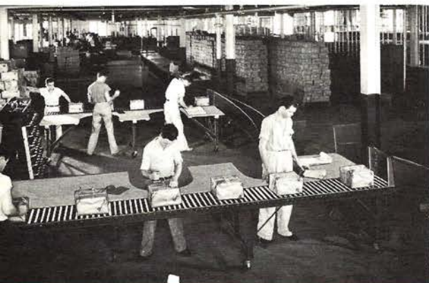
ABOVE: Battery of grinding machines served by Logan Roller Conveyor. Bearings in rolls are dust-protected type.
