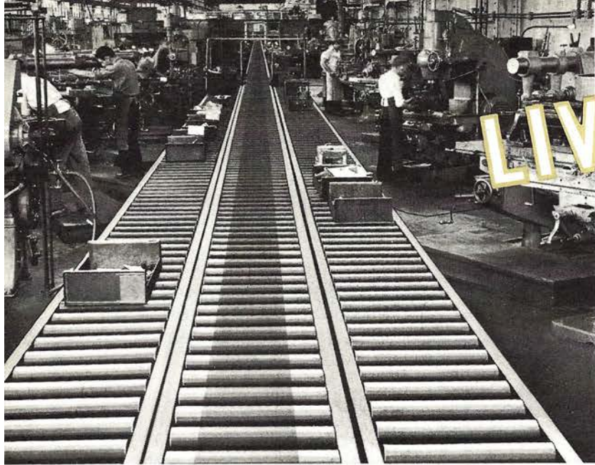
ABOVE: A Logan Live Roller Conveyor handling parts for electric motors and appliances between machine operations. Paralleled on either side by Roller Conveyor onto which the material is transferred while machine operations are performed.
