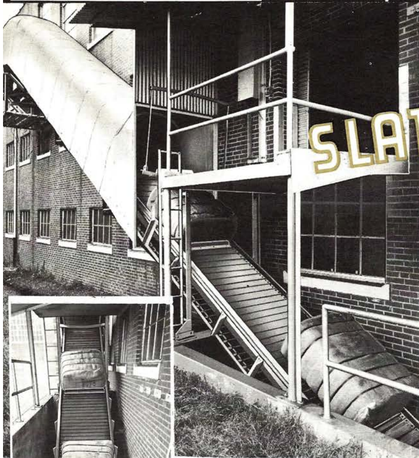
ABOVE: Logan Slat Conveyor handling bales of cloth from basement and first floor storage to finishing department on second floor. View at left shows basement feed end. Platform above serves first floor via hinged slide at entrance to housing. A roller conveyor curve facilitates discharge into building at second floor.
